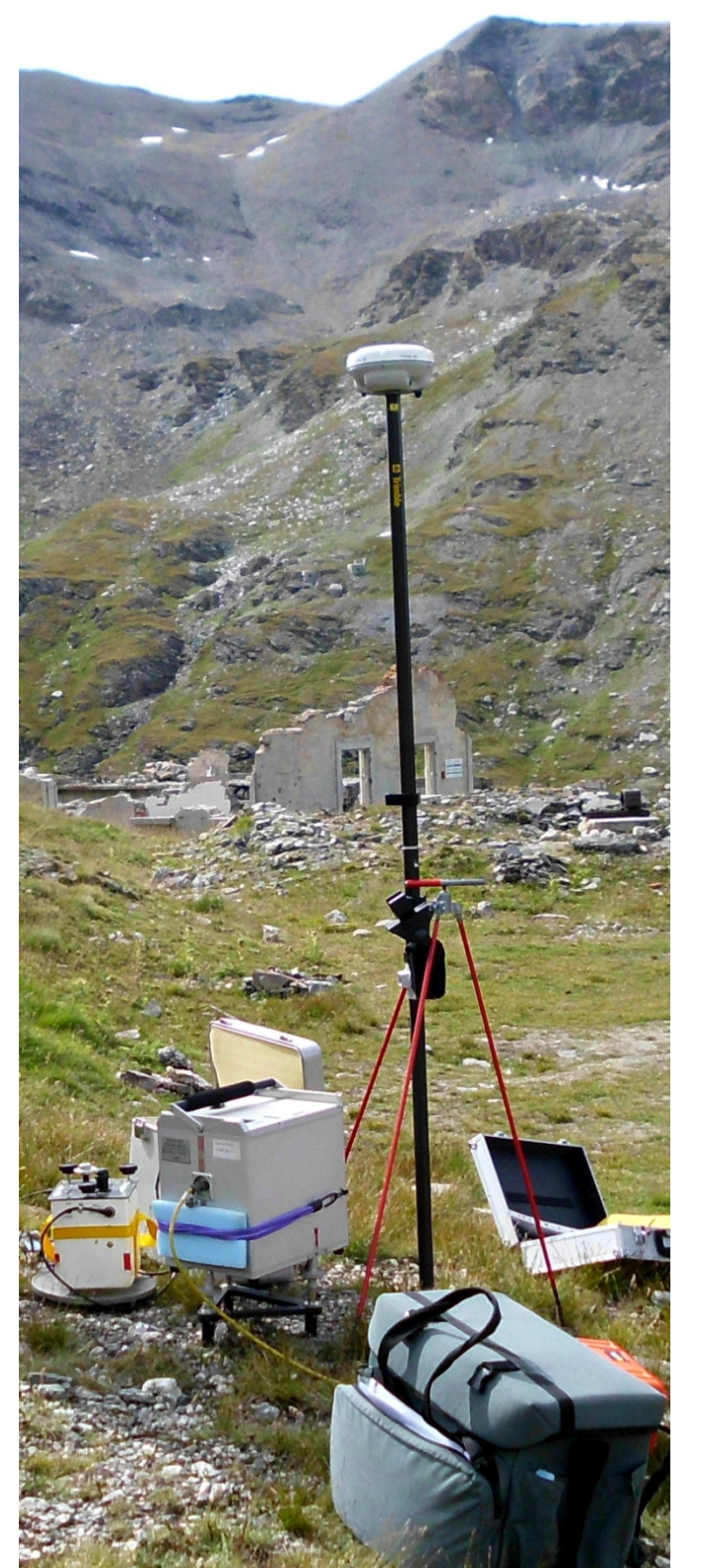
Relative gravimetry with field gravimeters and GNSS positioning
