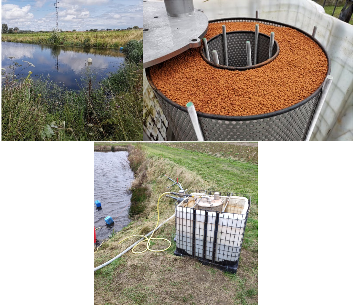
Figure 3. The upscaled P filter installed at Roeselare (Godelievegronden INAGRO)
