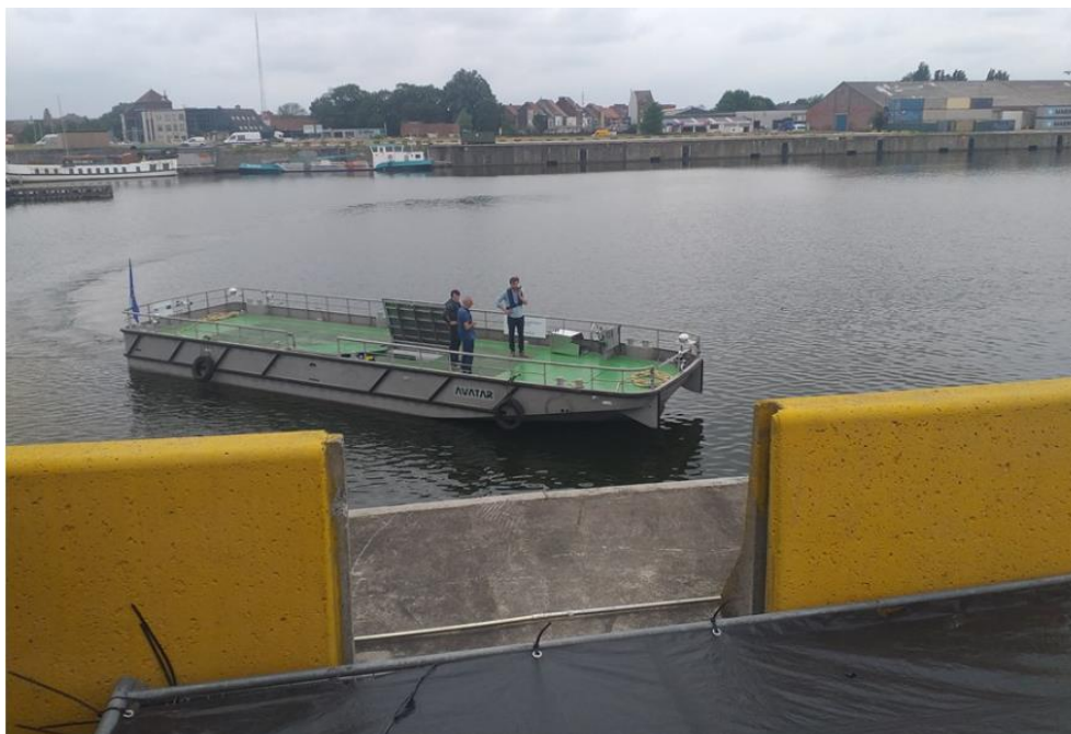
Figure 5: AVATAR-vessel sailing in Ghent, remotely controlled by SEAFAR from Antwerp
