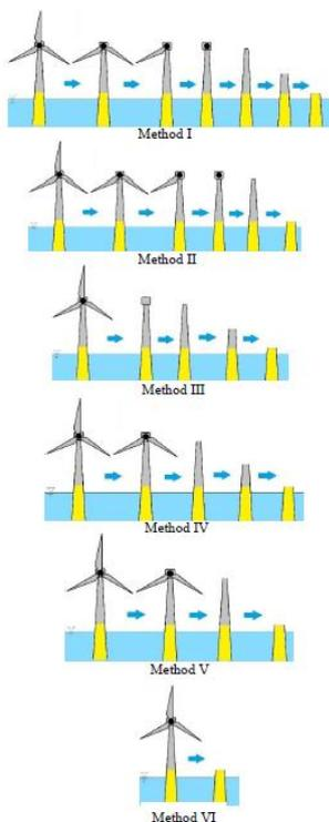
Figure 5: Decommissioning techniques offshore wind turbine
