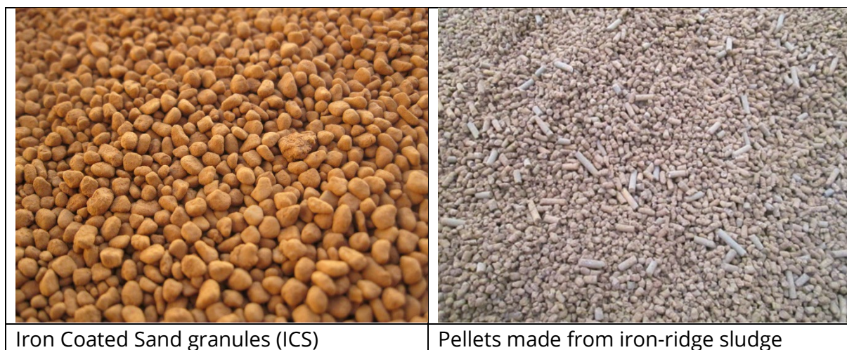
Photo 1 Iron Coated Sand granules (ICS) (left) and pellets made from iron-ridge sludge (right) at the start of the trial
