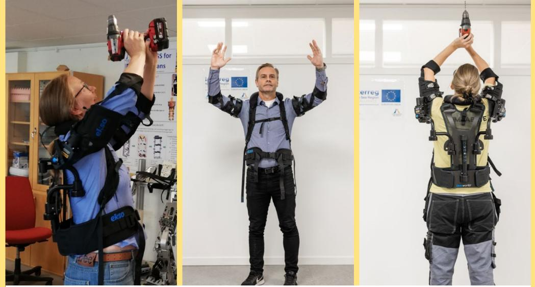
Overhead drilling operation with the EksoVest at University of Gävle
