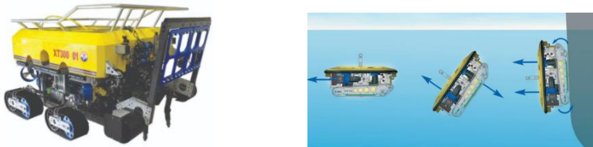
Figure 15 Bottom-crawler - XT300 [32] (to the left), Immersed structure crawler – Rovingbat (to the right) [28]
