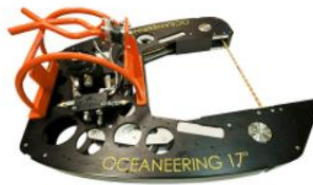
Figure 17 Diamond wire cutting tool [50]
