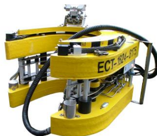
Figure 18 Abrasive water jet cutting tool [50]
