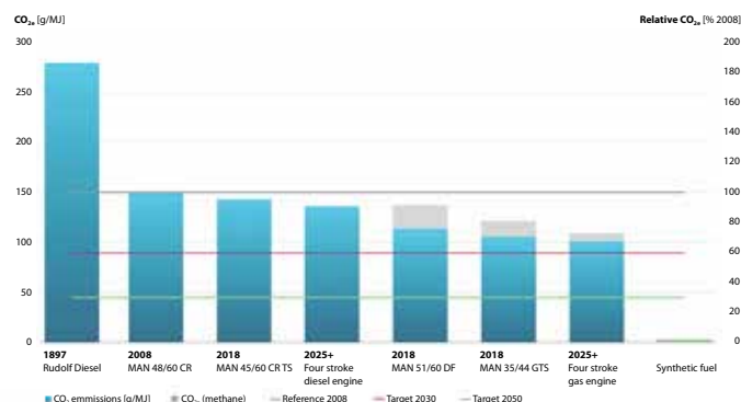
Figure 4. Comparison over time of \text{CO}_2 emissions from different types of MAN four-stroke engines – how low can it go?
