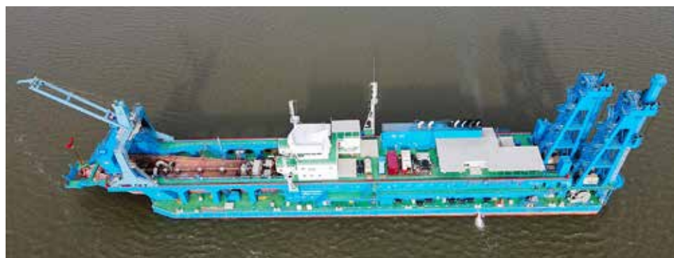
The non-propelled cutter suction dredger Mohab Mameesh (photo A. Neighbourfield).
