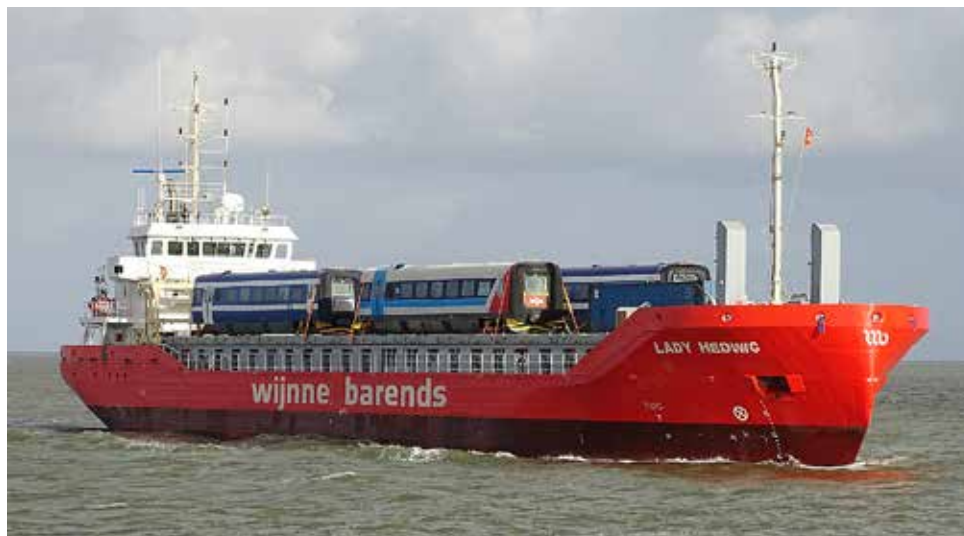
The Lady Hedwig is the third in a series of six ice class 1 A multipurpose vessels (photo F.J. Olinga).
