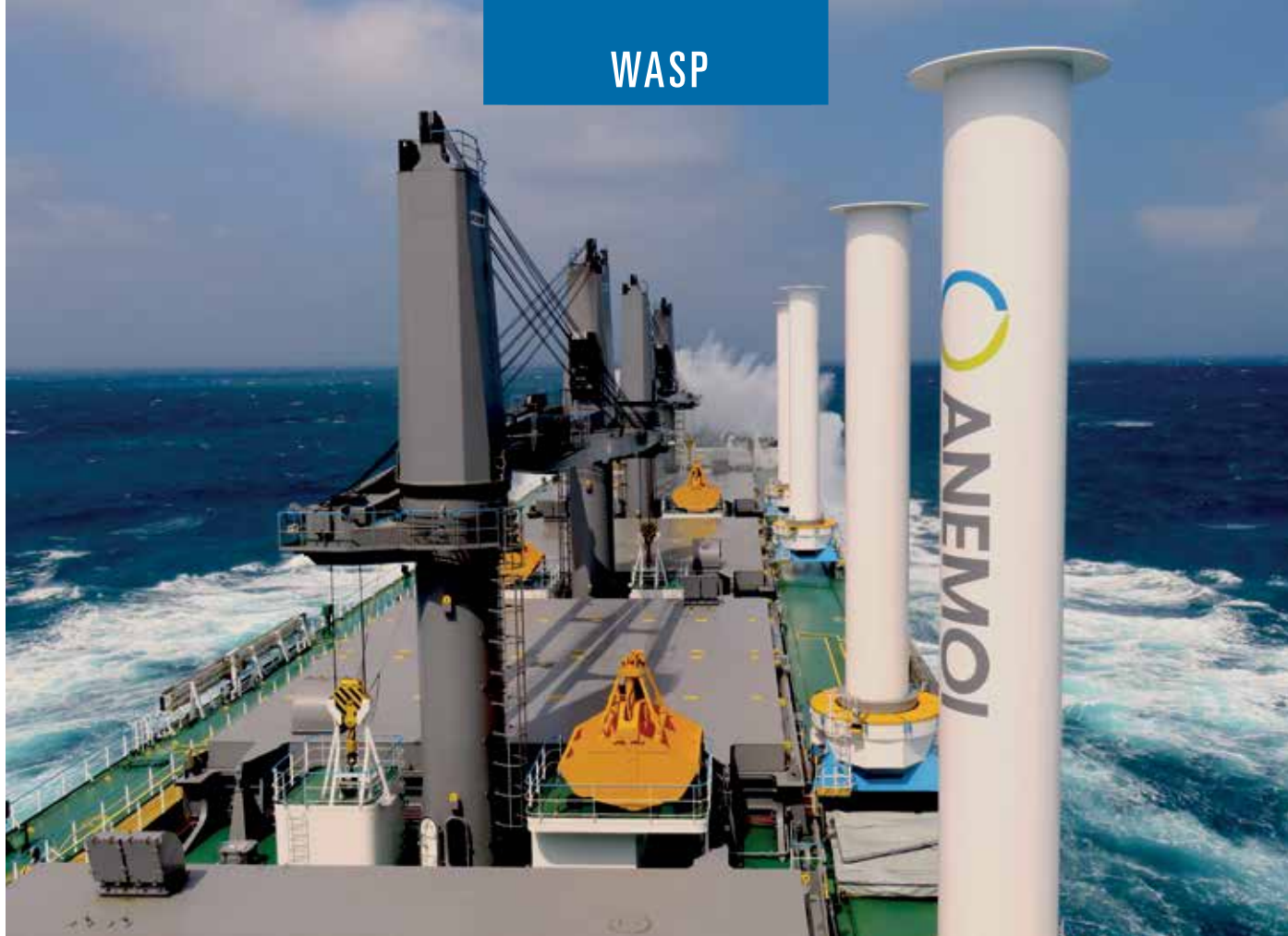
The Ultramax bulker Afros carries four movable rotors.
