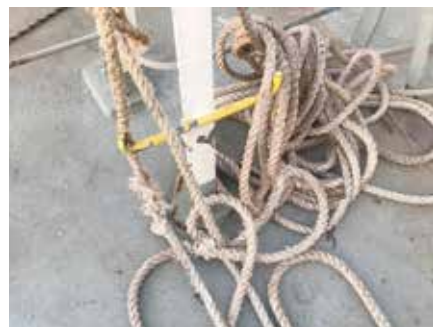
All of the safety lines appeared in poor condition.
