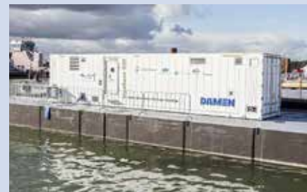
The Damen containerised ballast water treatment system InvaSave offers a port-based solution to ships ill-equipped to treat their ballast water.
