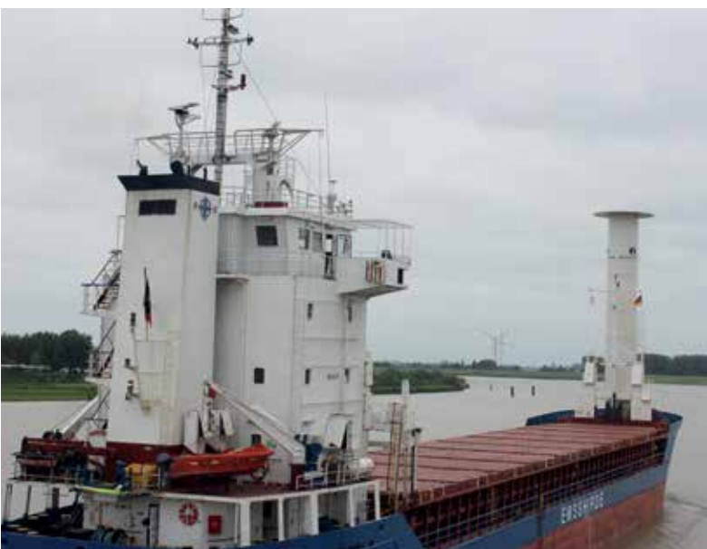
The Fehn Pollux is retrofitted with one rotor.
