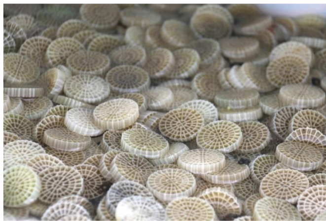
Photo 2: Plastic carriers in a MBBR, on which a biofilm will develop
