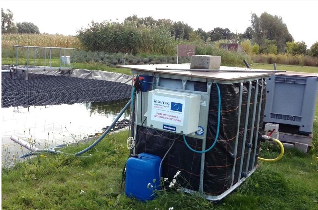
Photo 1: Set-up of Moving Bed Biofilm Reactor (MBBR) at PCS Ornamental Plant Research
