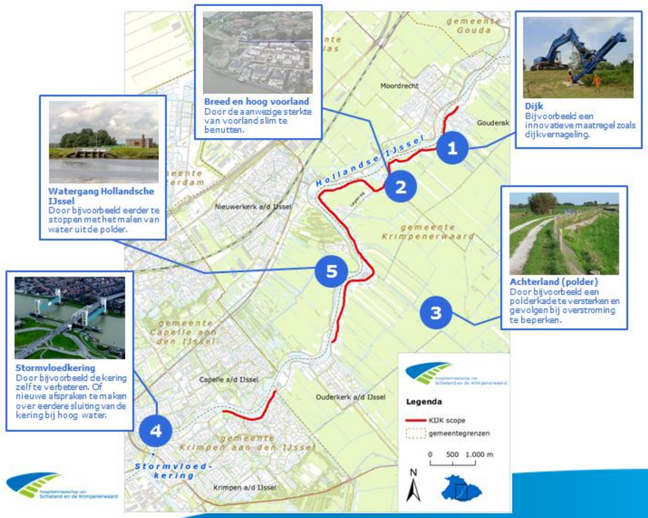
Figure 5: The whole system approach of finding solutions for the functional goal of project KIKJ.
