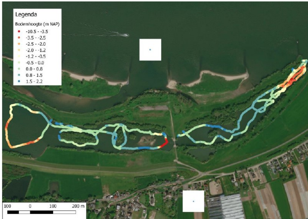
Figure 4: Tracks and measured depth, using the vessel and the fishfinder.
