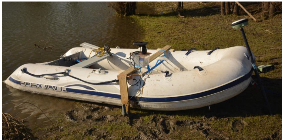
Figure 2: equipment needed for the measurements. The Fishfinder is visible mounted on the vertical shelf.
